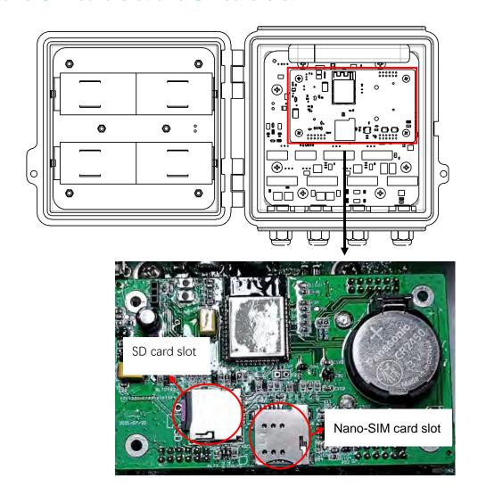
MC-BW-B meter controller is equipped with Nano-SIM card slot and SD card slot (using TF memory card). Insert the Nano-SIM card, the controller will automatically connect to the network and upload the data to the cloud platform. Upload to the company's cloud platform by default. To switch to other data platforms, please check the configuration information. The controller comes standard with a 32 GB memory card.
