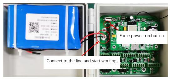
The battery power supply adopts intermittent working mode. The user can set the normal power-on time and standby sleep time. Users can set it according to their needs.
