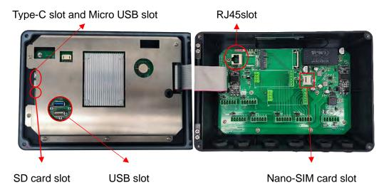
MC-W-S is equipped with Nano-SIM card slot and SD card slot. Insert the Nana-SIM card, the MC-W-S will automatically connect to the network and upload the data to the cloud platform. By default, the company's cloud platform is uploaded. To switch other data platforms, please check the configuration information. MC-W-S comes standard with a 32 GB SD card.
